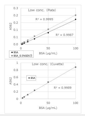
Calibration curves using low-concentration measurements These calibration curves were prepared using a 1/2 dilution series of the BSA standard. BSA and BSA containing 0.5% SDS (BSA\_0.5%SDS) were measured in a 96-well plate (top) and cuvette (bottom). It demonstrates that quantification is linear even in the low-concentration range.
